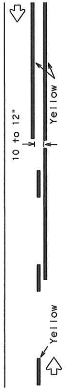
REFLECTORIZED PAVEMENT MARKINGS - PATTERN A
