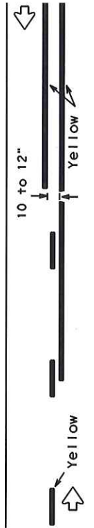
REFLECTORIZED PAVEMENT MARKINGS - PATTERN A
